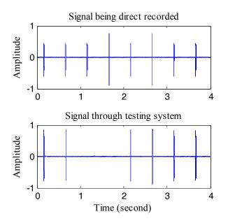
Figure 2 Loss of pulses in audio processing path at low latency setting
