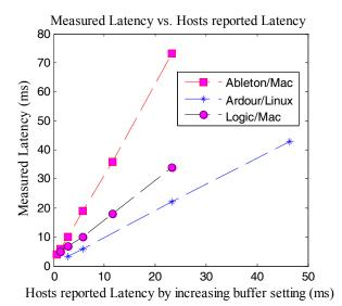
Figure 3 Measured Latency vs. Hosts reported Latency in millisecond with different buffer setting
