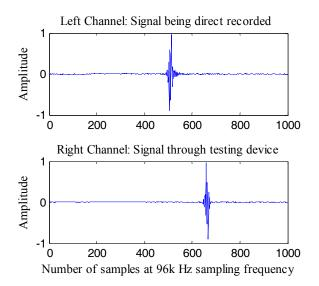
Figure 1 Latency measurement from recorded signals
